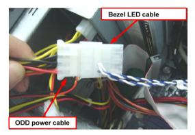
9. Pull out the master ODD data cable and power cable.
